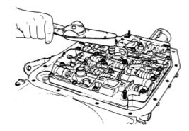
Reinstall the oil pan using the supplied gasket or the OEM reusable unit . Tighten the bolts to 10 foot/pounds. Refill the transmission in a known fashion. Recommend fill with 4 quarts, start engine, continue fill to full. *DO NOT OVERFILL TRANSMISSION!* After first road test recheck transmission for leaks and proper fluid level.
